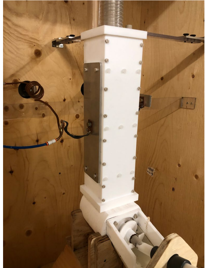
The vertical applicator (reactor) used in the RF process.
