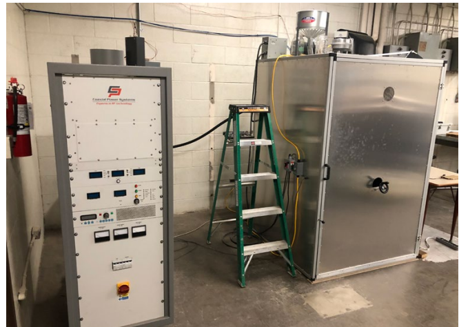
The complete RF system, including generator (left) and the vertical applicator with the container door closed (right).
