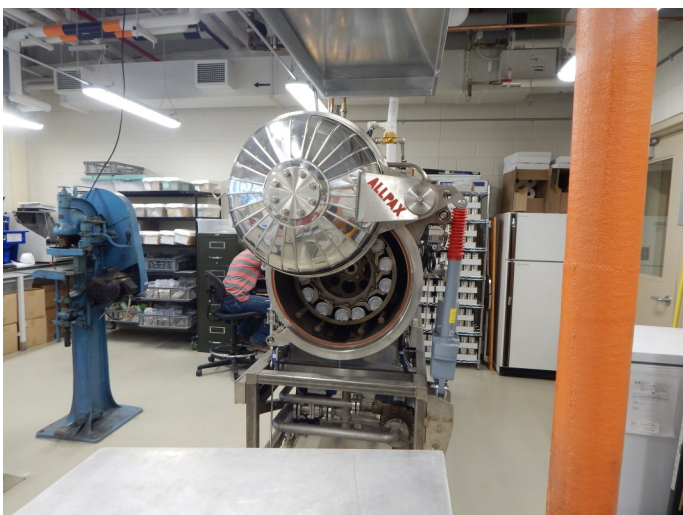
The Rotary Canner at Bean Pilot Plant at the AAFC Lethbridge Research and Development Centre was purchased a number of years ago with grower funds leveraged through the Pulse Science Cluster.
